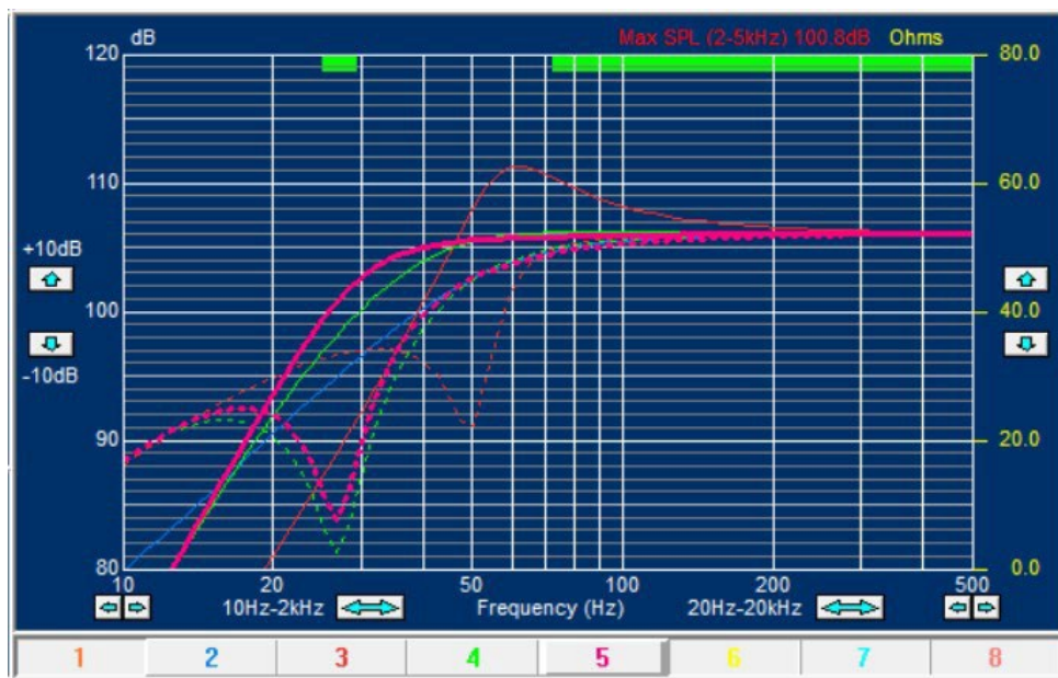
Figure 22 - Four different Bass Reflex Simulations
