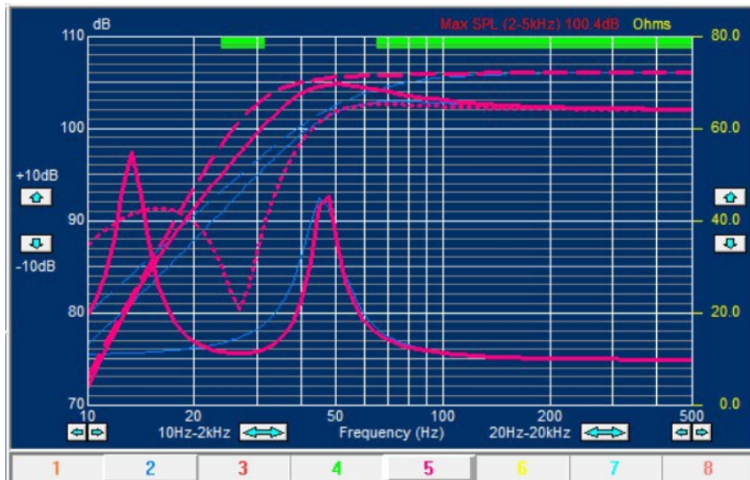
Figure 23 - High Power Bass Reflex versus Closed Box
