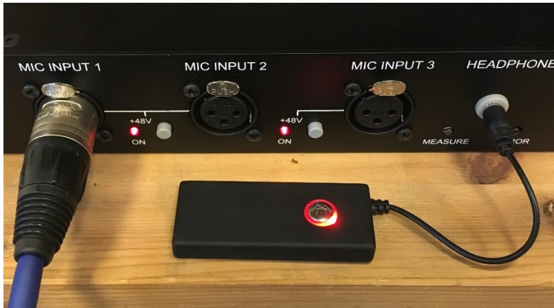
Figure 49 - Bluetooth Transmitter connected to Headphone output
