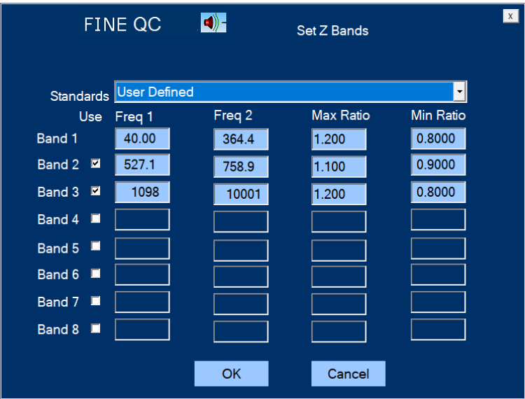
Figure 38 - Impedance Limits Setup
