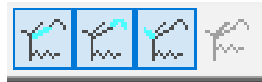
Figure 28 - Include or exclude the contribution of different parts of the model in the frequency response
