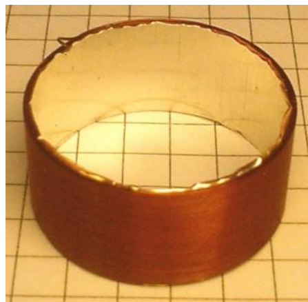
Figure 41 - The voice coil used in the woofer we are simulating
