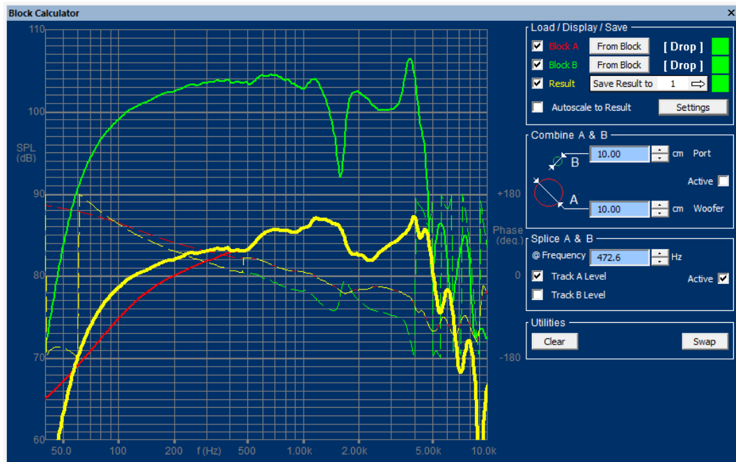
Figure 29 - Far and near-field curves spliced at 472.6 Hz
