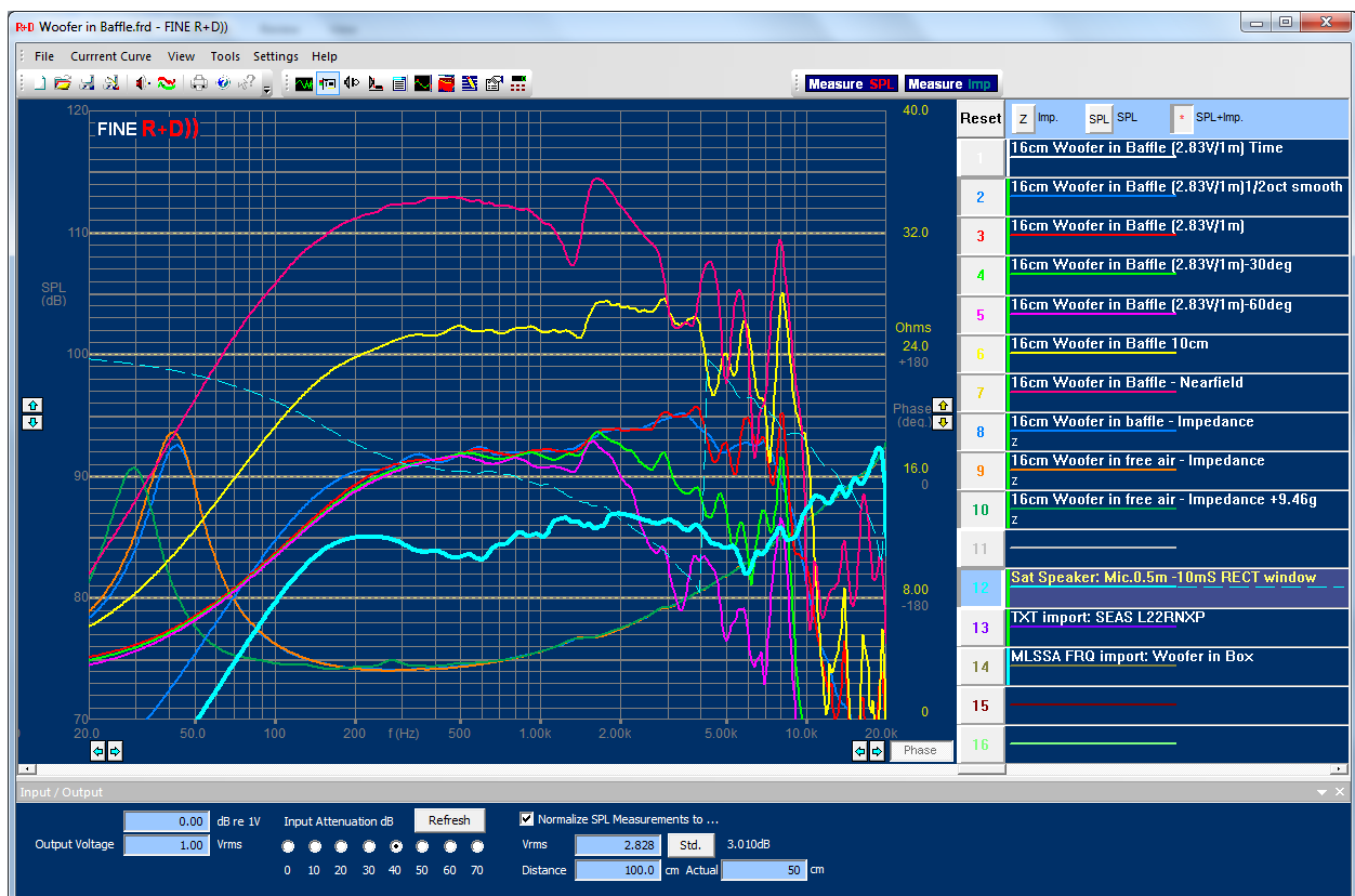
Figure 16 - Satellite speaker measured at 0.5m and normalized to 2.83V/1m (cyan curve #12)
