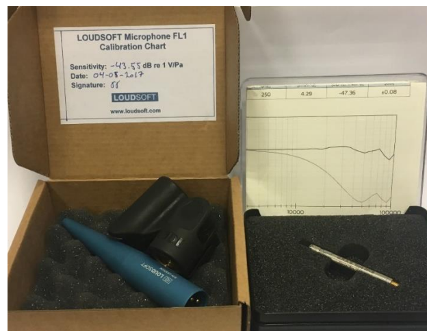
Figure 2 - Microphone sensitivity charts. Left is the LOUDSOFT FL1 microphone and right is the GRAS 46BE microphone.
