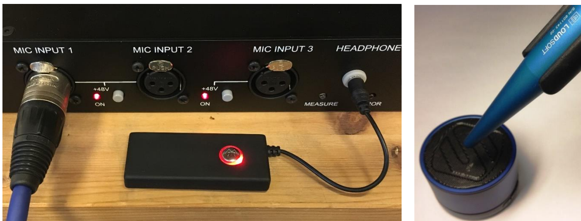
Figure 60 - Bluetooth transmitter connected to Headphone output, which is in parallel with the Line Out.
