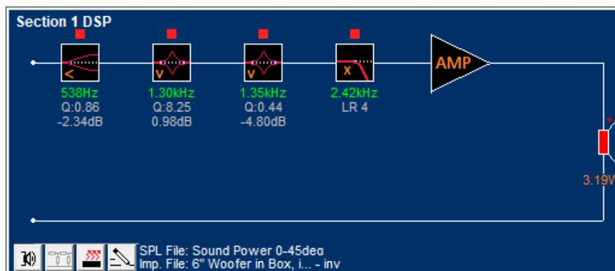
Figure 18 - DSP blocks with Freq, Q and level (dB)
