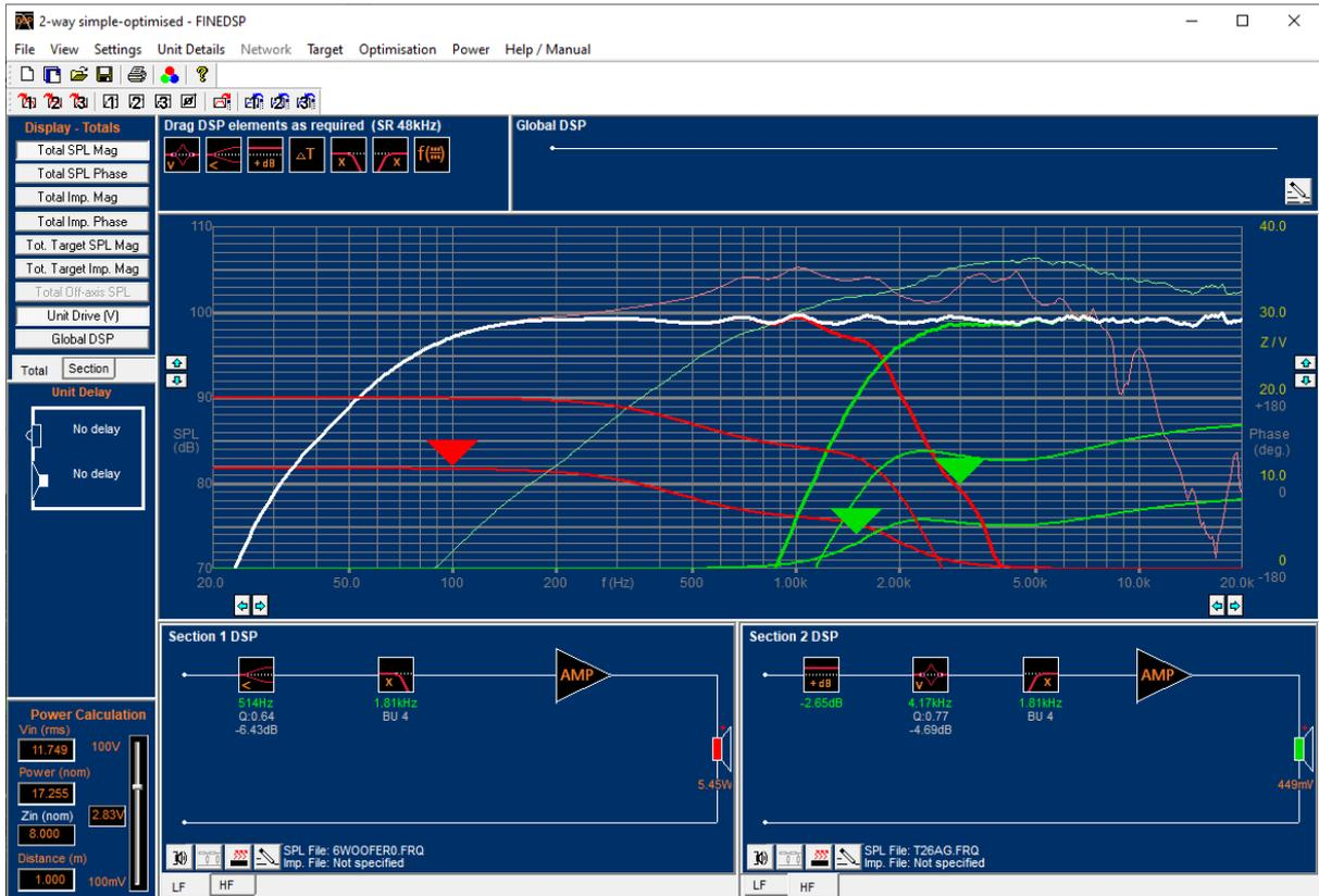
Figure 11 - FINE DSP main display for the simple 2-way X-over, with red & green power arrows
