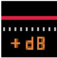
The level control can adjust the level by a specified amount of +/- dB. This feature is useful for adjusting the level of a tweeter, which is often more sensitive than the woofer in a system.
