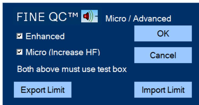
Figure 44 - Select "Micro Test" for Enhanced Rub & Buzz
