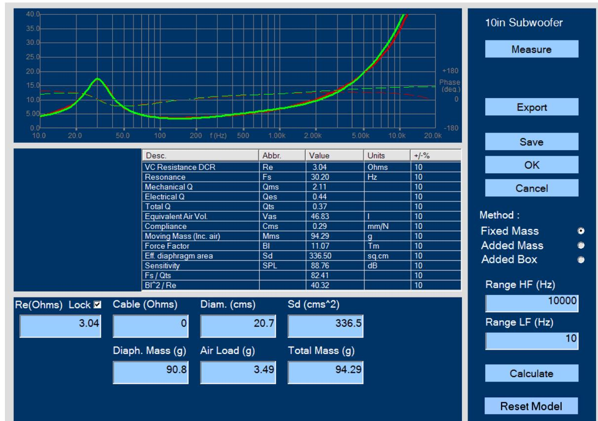
**Figure 45 - TS Parameters of 10-inch Subwoofer**
