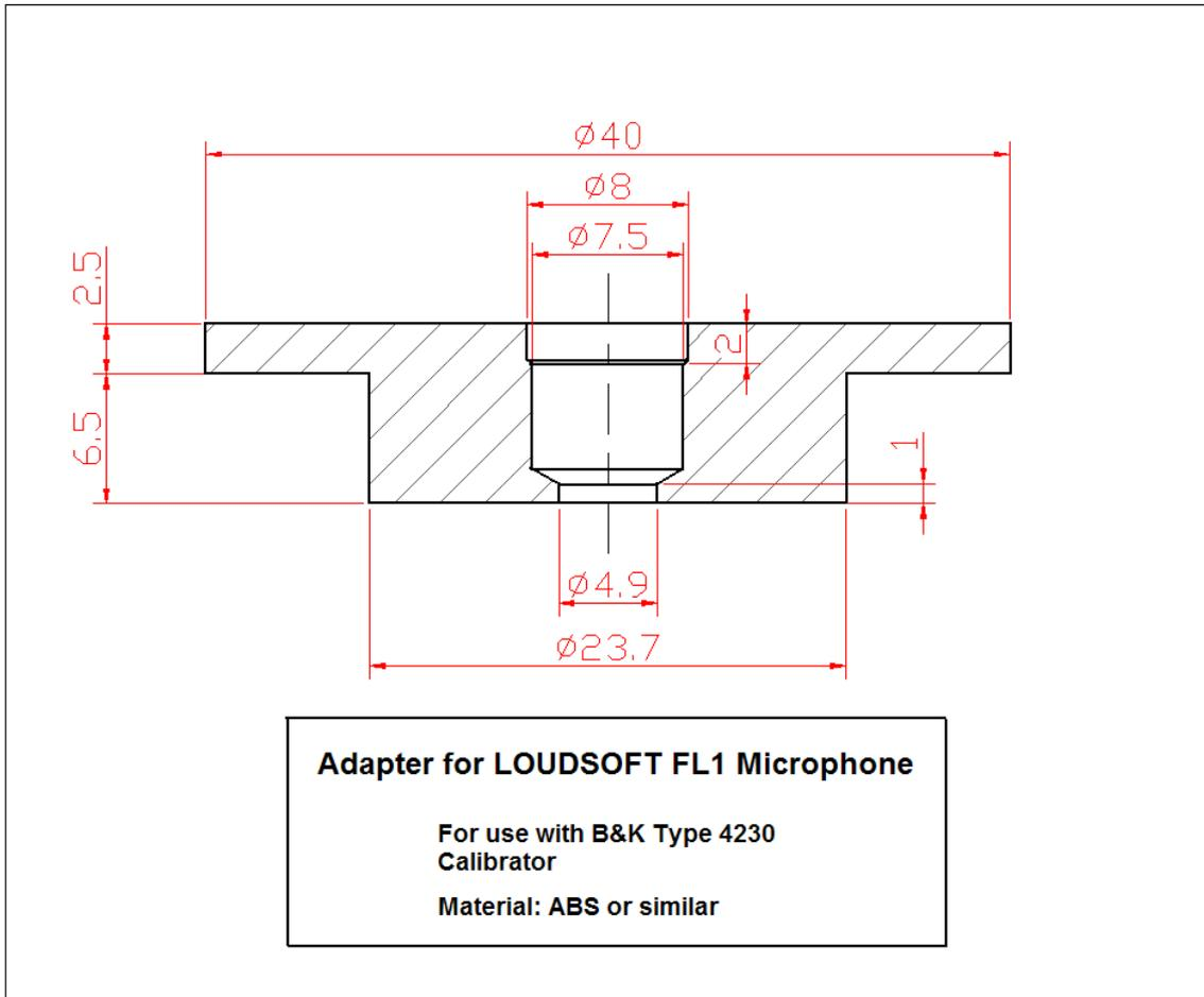
Figure 68 - Adapter for FL1 Microphone
