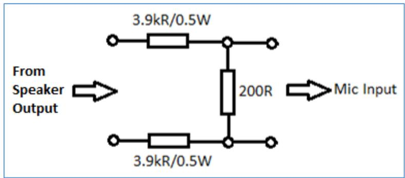
Figure 51 - Attenuator for High Power Amp Test. Max V=40V input (=400W/4R)
