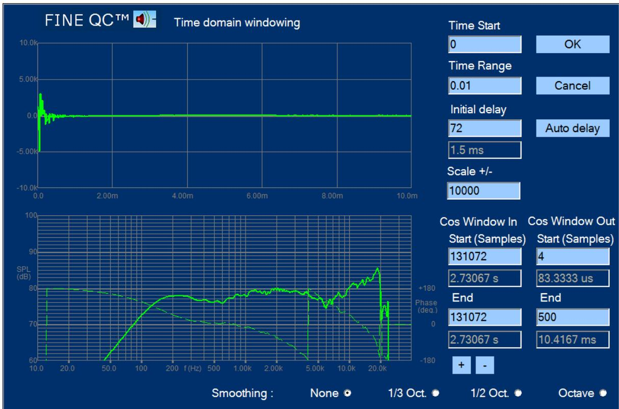
**Figure 36 - Satellite and Microphone moved 154cm above floor, Microphone Distance 0.5m**
