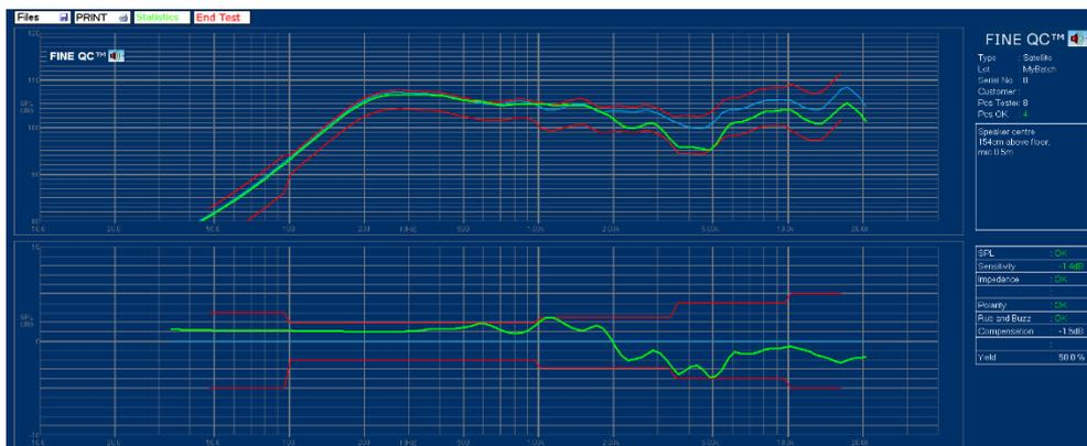
Figure 26 - SPL Statistics with Adjusted Limits
