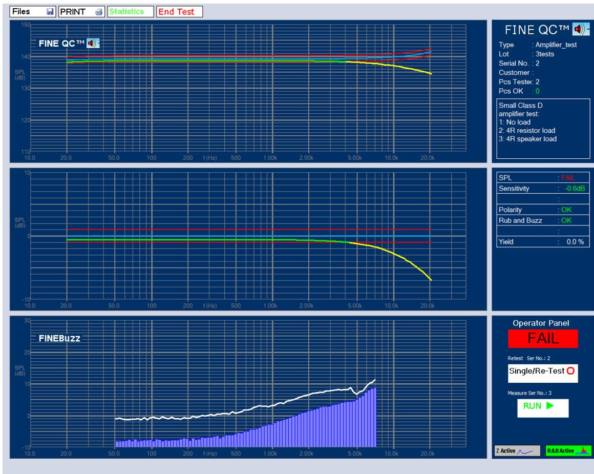
Figure 53 - Amplifier Test: #2 failed due to 4R load
