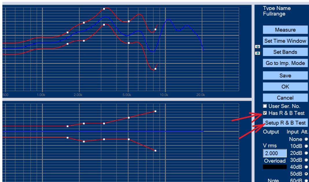
Figure 16 - FINEQC can also measure Rub and Buzz which must be specified in the specifications window
