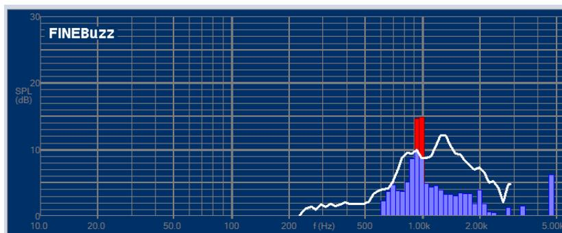
Figure 41 - Tweeter with Very Subtle Buzzing Tinsel at 900Hz
