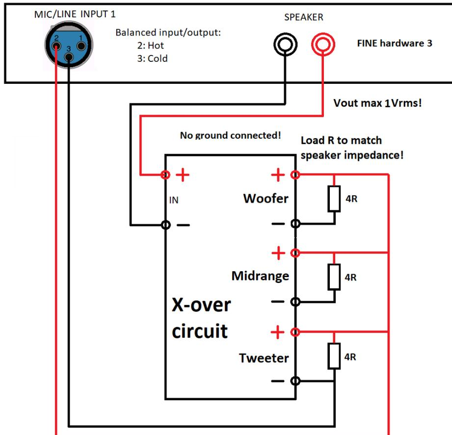
Figure 49 - QC test of X-over (Cross-over) circuit. Remember load resistors
