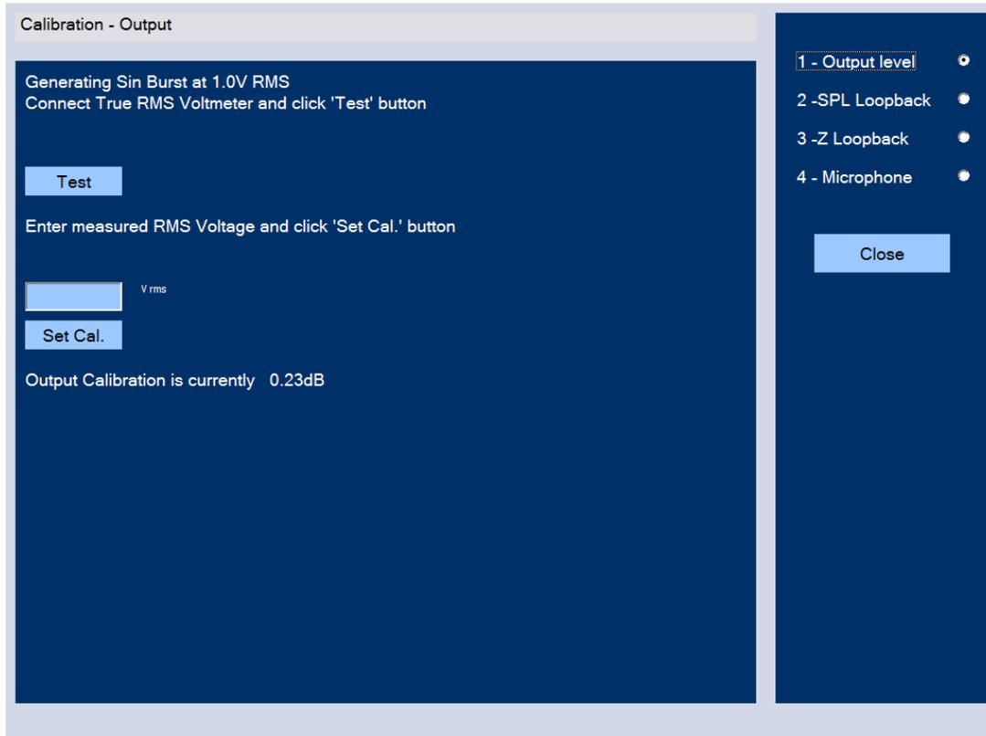
**Figure 59 - The output level calibration window**
