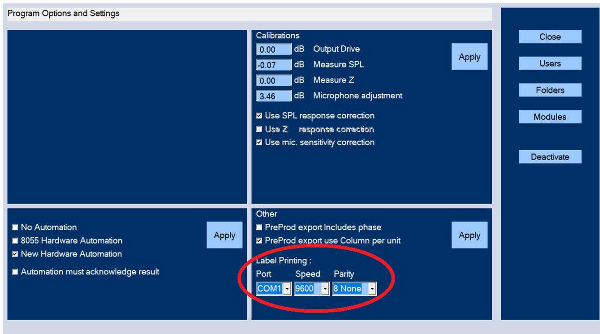
Figure 55 - The printing options can be changed in the admin panel
