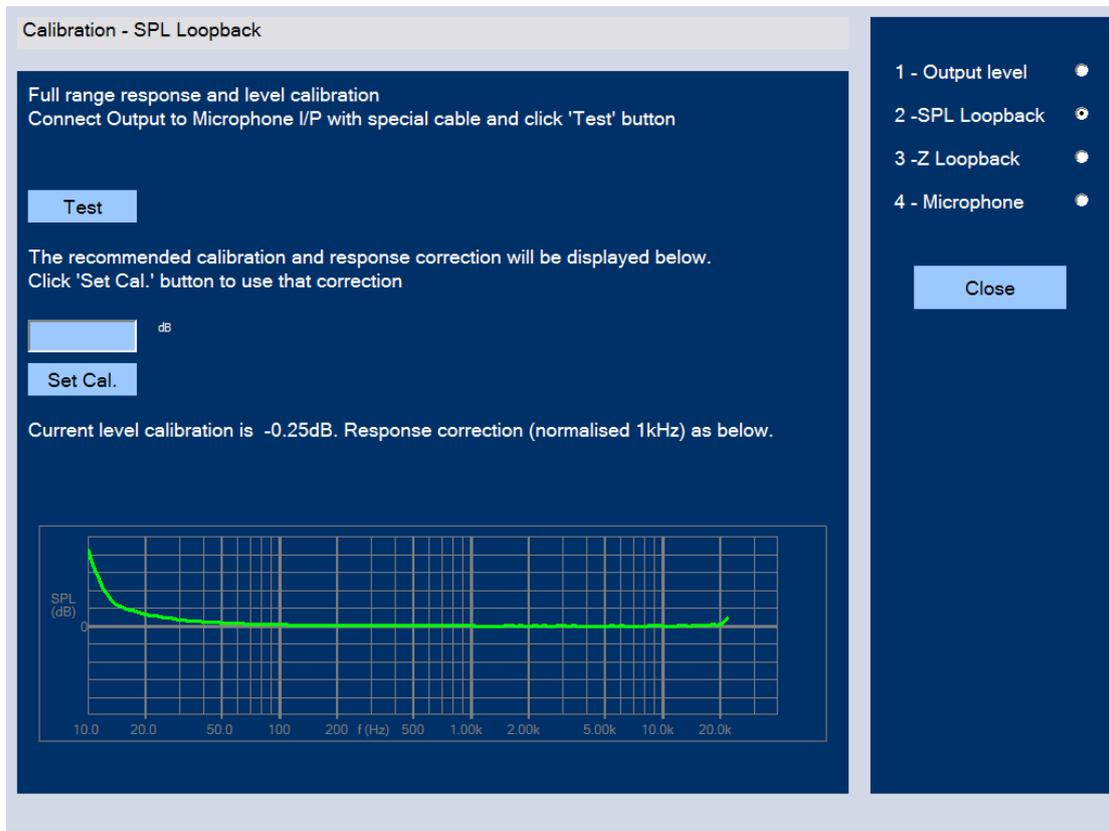
**Figure 60 - The SPL loopback calibration window**
