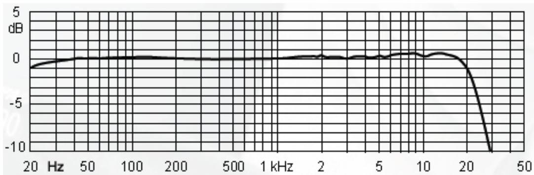
Figure 67 - On-Axis Frequency Response of LOUDSOFT Microphone FL1 in Free Field
