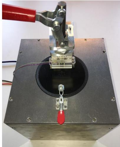
**Figure 69- LOUDSOFT Aluminum Test Box –small**
