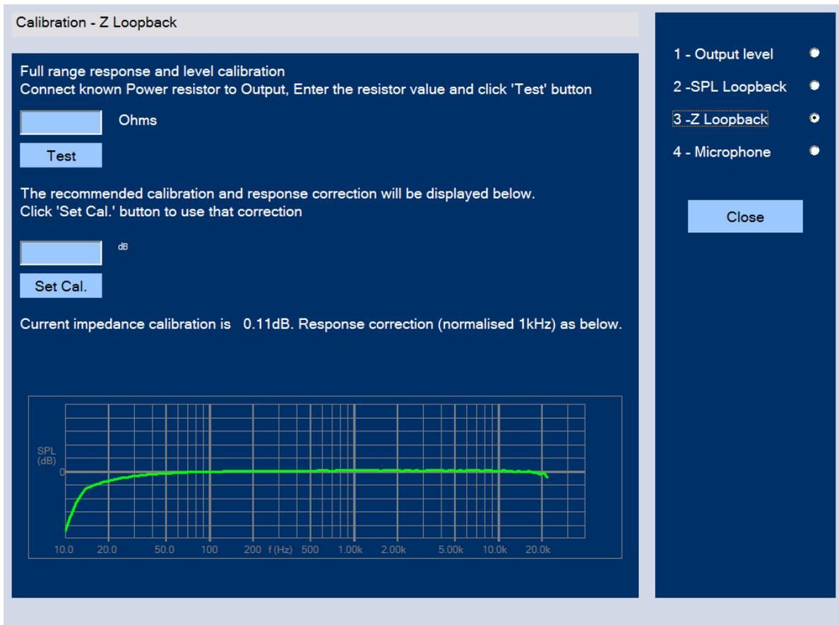
Figure 62 - The impedance loopback calibration window
