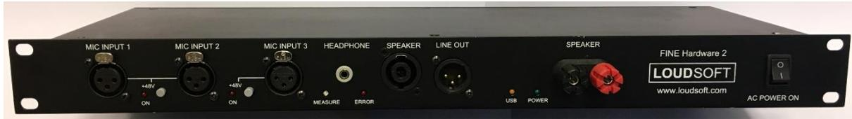
Figure 64 - The front panel of the FINE Hardware 3
