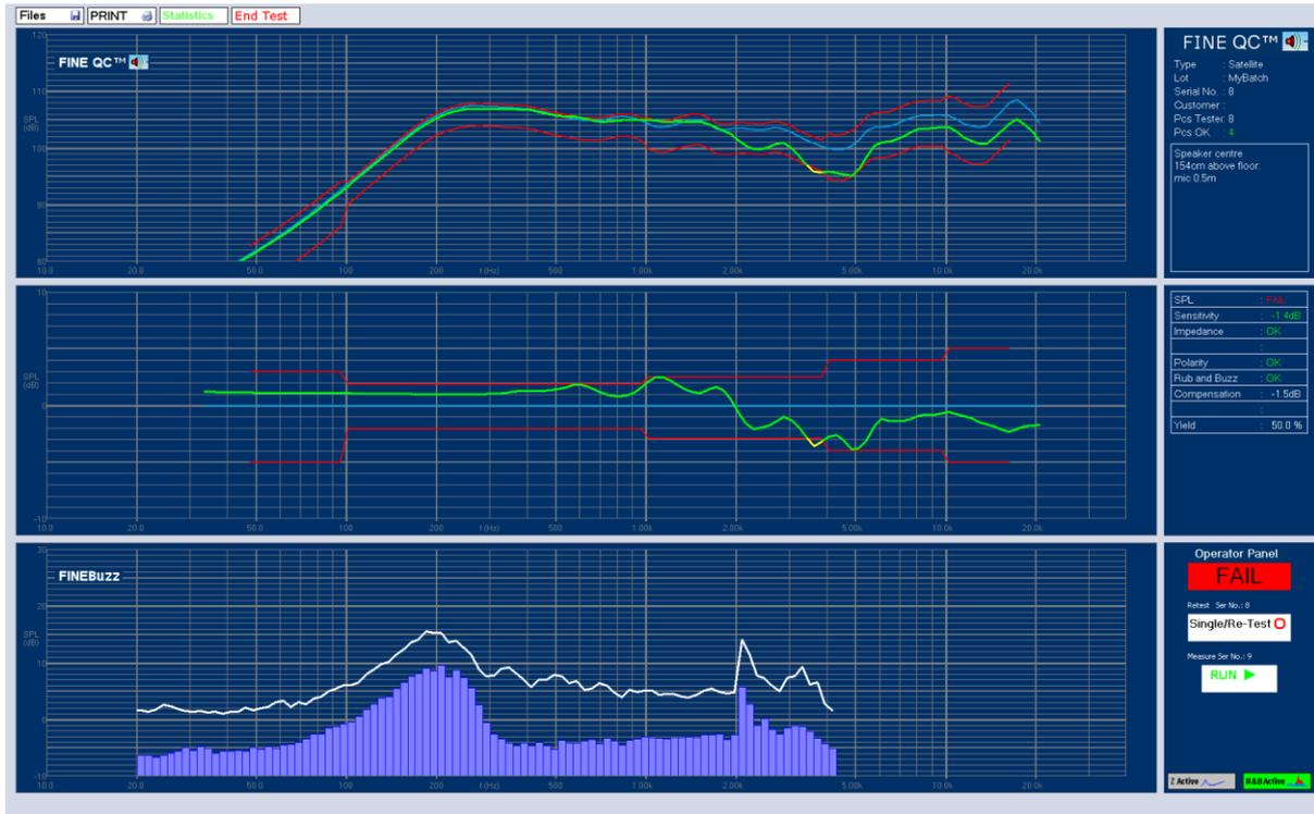
**Figure 20 - FINE QC Test Display: SPL FAIL at 3.5 kHz**
