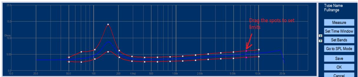
Figure 11 - It is possible to edit the limits by clicking and dragging the white dots
