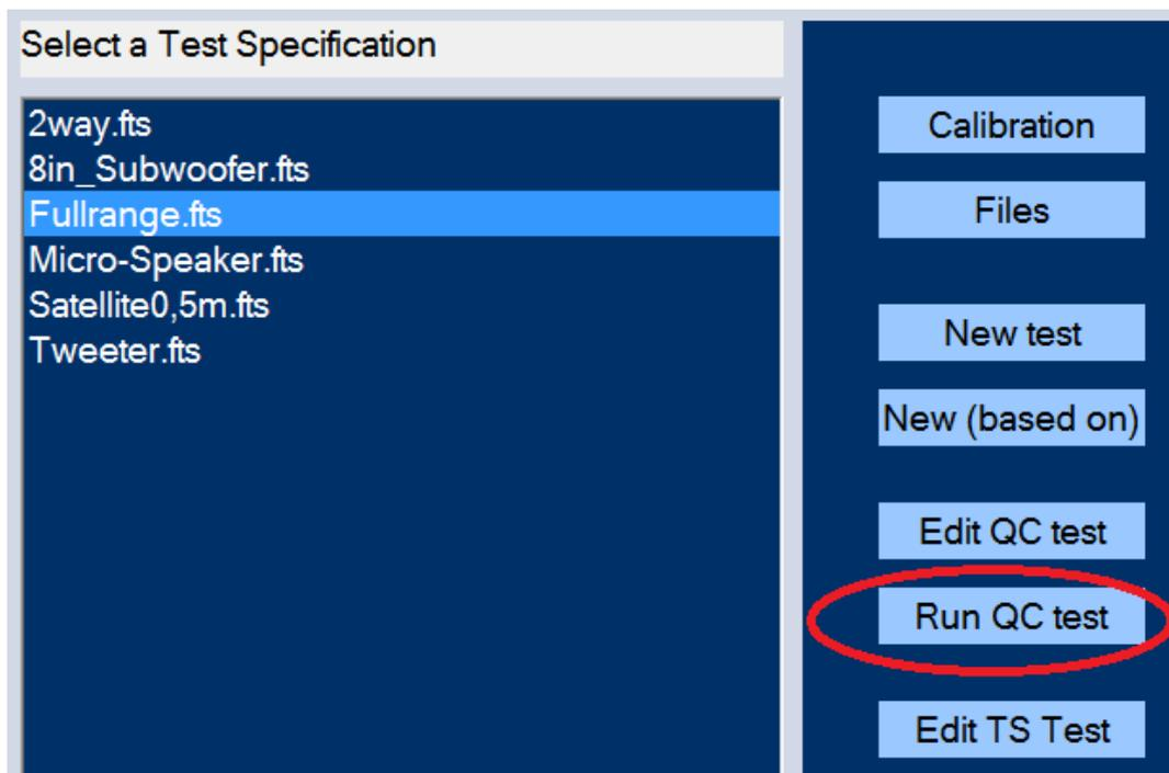
Figure 12 - When the test specifications have been set the test can be run from the main window
