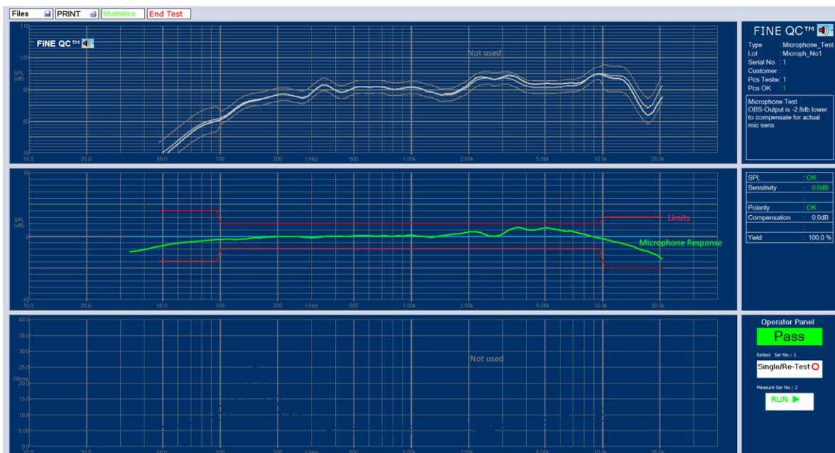
Figure 54 - Microphone response w limits tested with FINE QC
