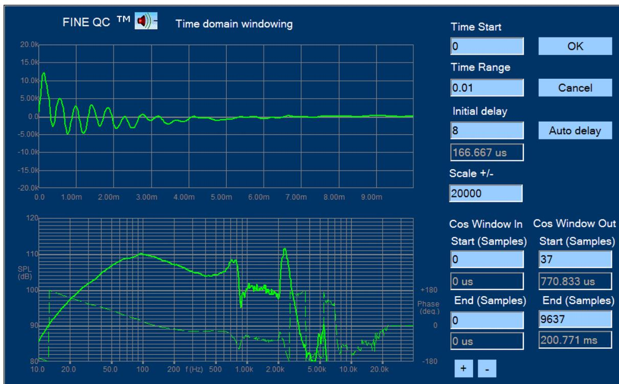
Figure 37 - 8-inch Woofer Measured in Near Field
