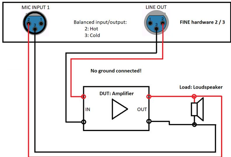
Figure 50 -- Electronics Testing: Amplifier connection diagram
