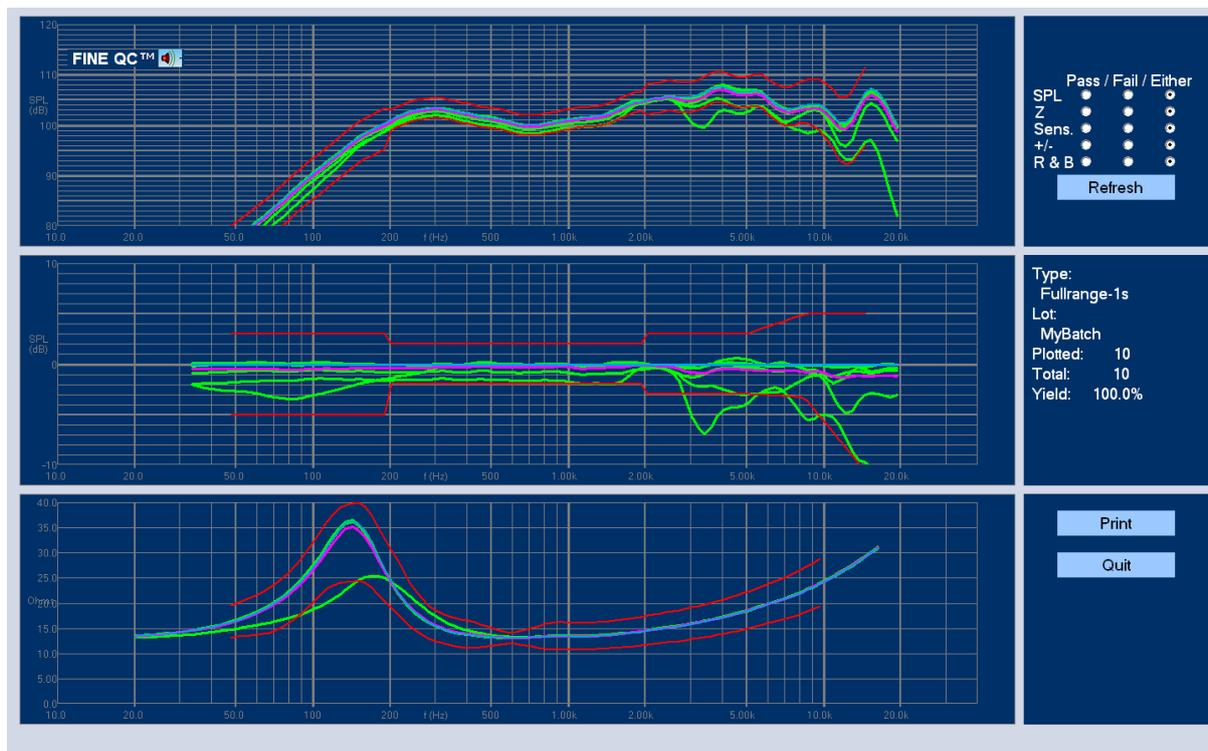
**Figure 18 - Statistical Result of Previous QC Test Series**
