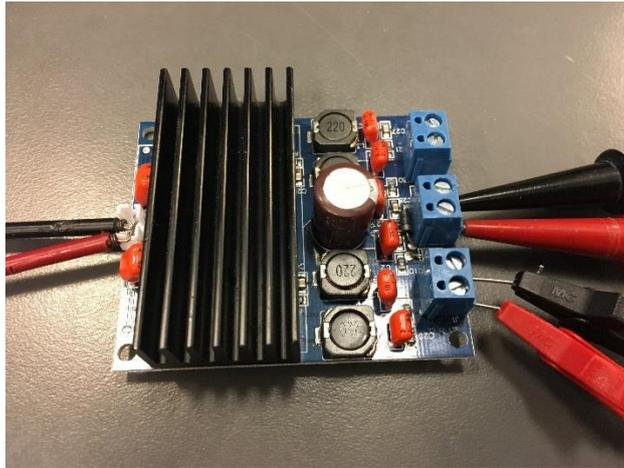
Figure 52 - Small (Class D) amplifier measured with FINE QC
