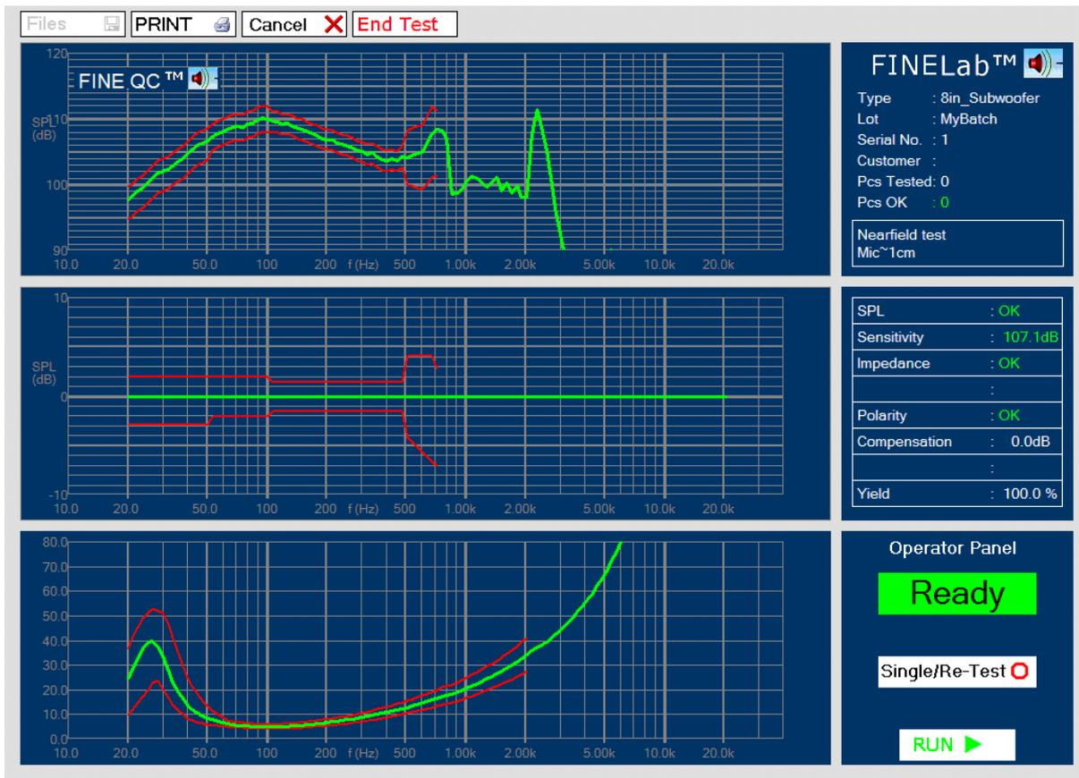
Figure 38 - 8-inch Subwoofer Test in Near Field
