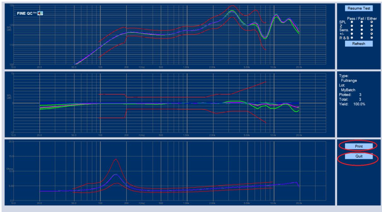
Figure 15 - When the test is done you can select what measurements you want to see and print them. You can view detailed info and responses in Pre-Prod, see Figure 18.
