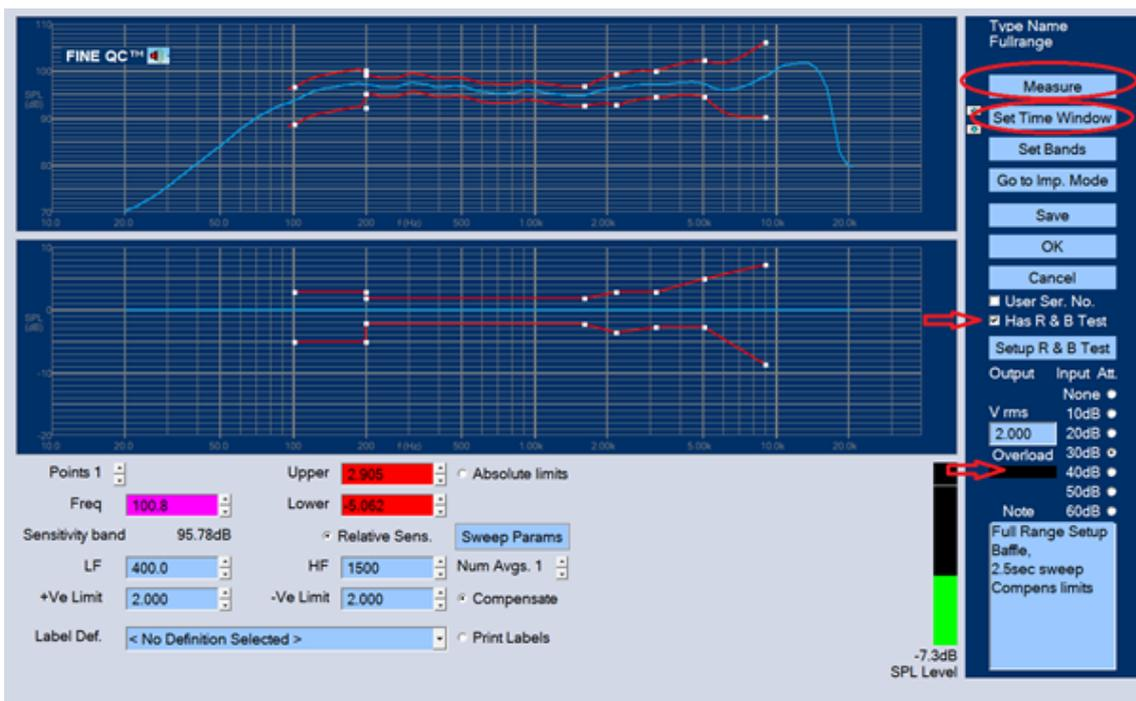
Figure 9 - Main window for editing test specifications
