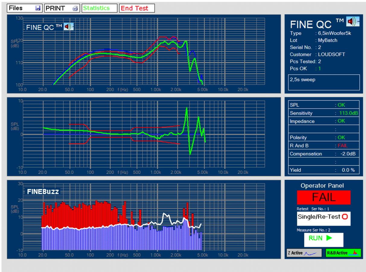
Figure 40 - 6.5-inch Woofer with Rubbing Voice Coil Found with FINEBUZZ
