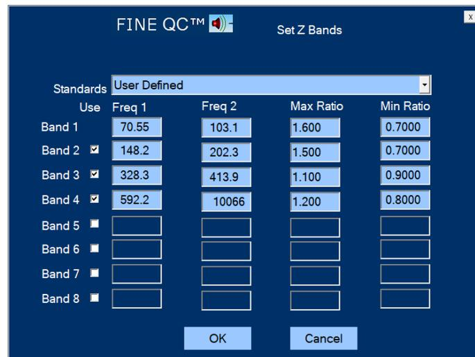
**Figure 28 - Full-Range Impedance Template**
