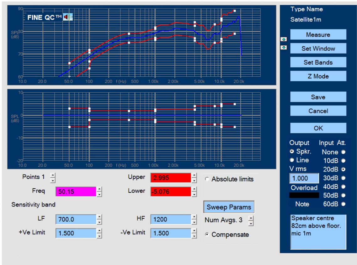
Figure 32 - Satellite Speaker Tested in Normal Room at 1m
