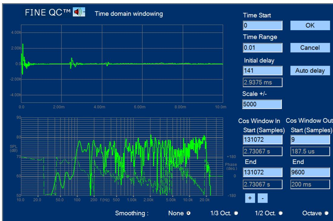
**Figure 34 - Time Response of Satellite at 1m Microphone Distance and 82cm above Floor**
