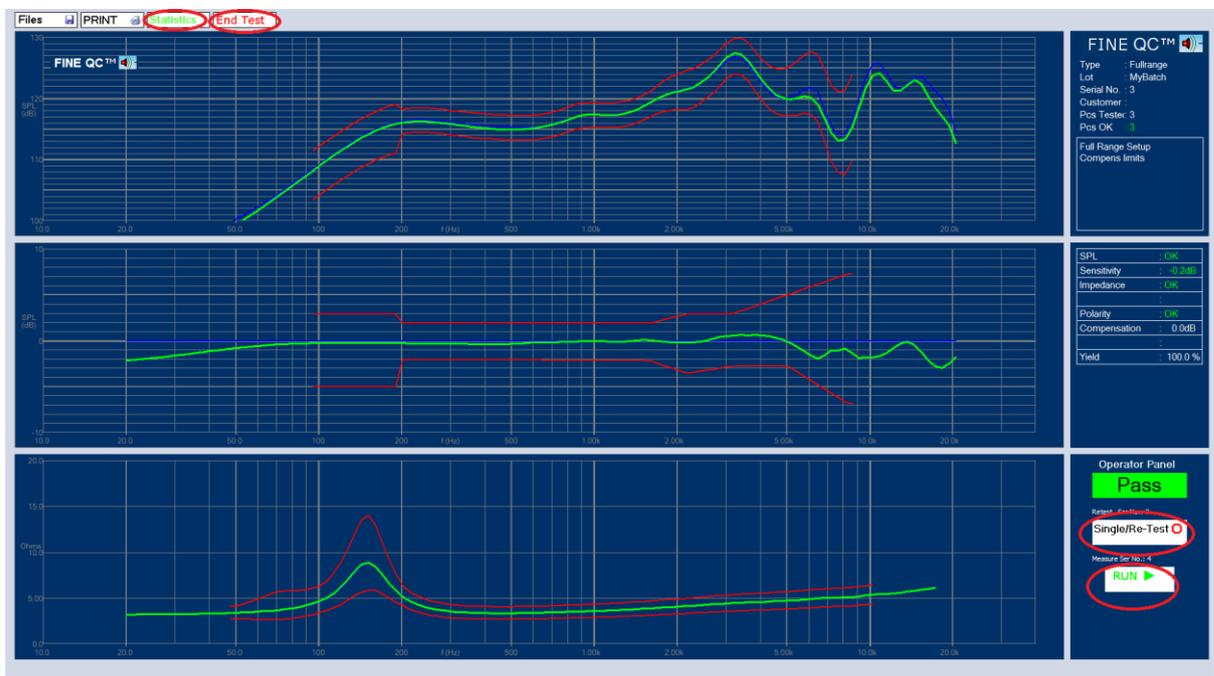
Figure 14 - In the main measuring window the frequency response, the deviation from the reference (center) and the impedance can be seen
