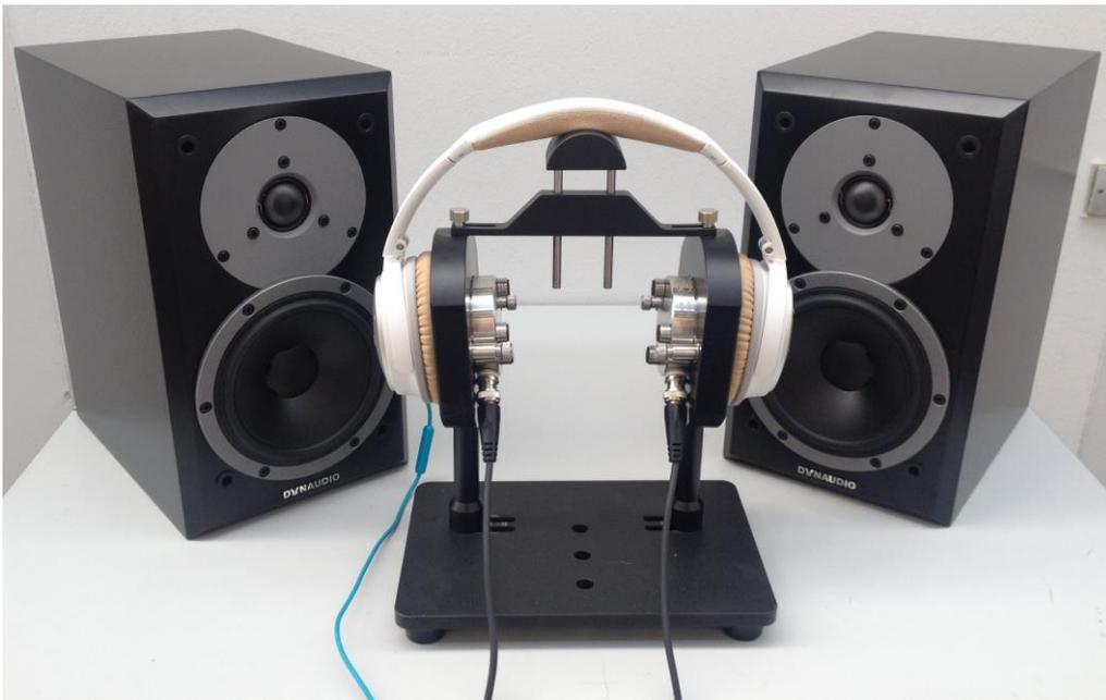
Figure 2 – Noise Cancel Testing using two Dynaudio Emit M10 speakers
