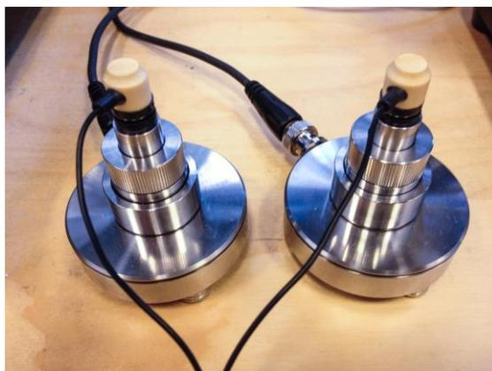
**Figure 35 - CRY IEC318 Artificial Ear Simulators for in-ear headphone testing**
