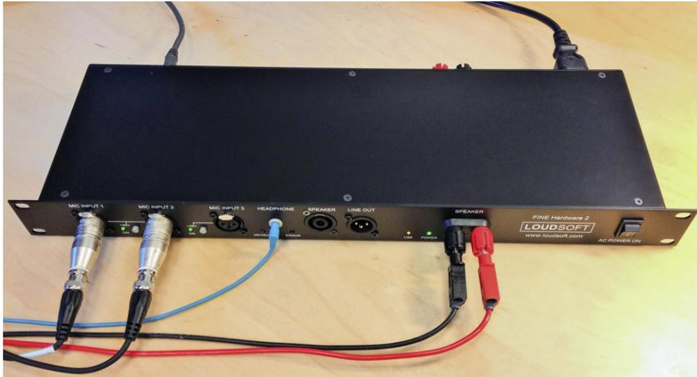
**Figure 1 - FINE Hardware 2 for measuring headphones, including Noise Cancel test.**
