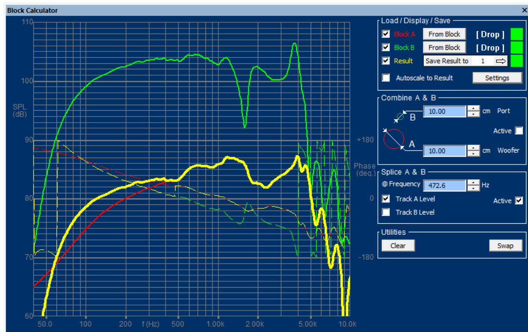
Figure 19 - Far and near-field curves spliced at 472.6 Hz
