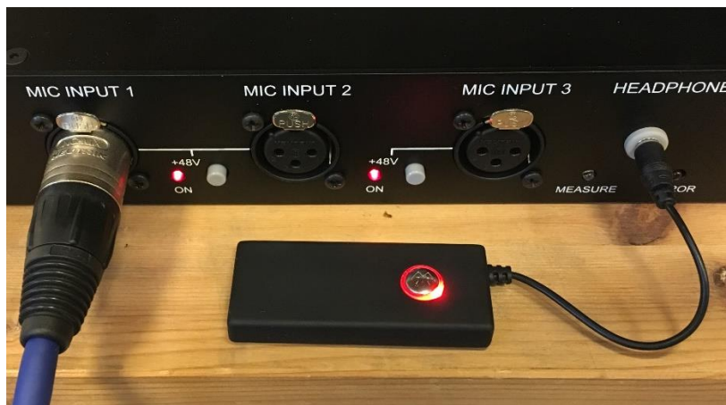
Figure 48 - Bluetooth transmitter connected to Headphone output, which is in parallel with the Line Out.
